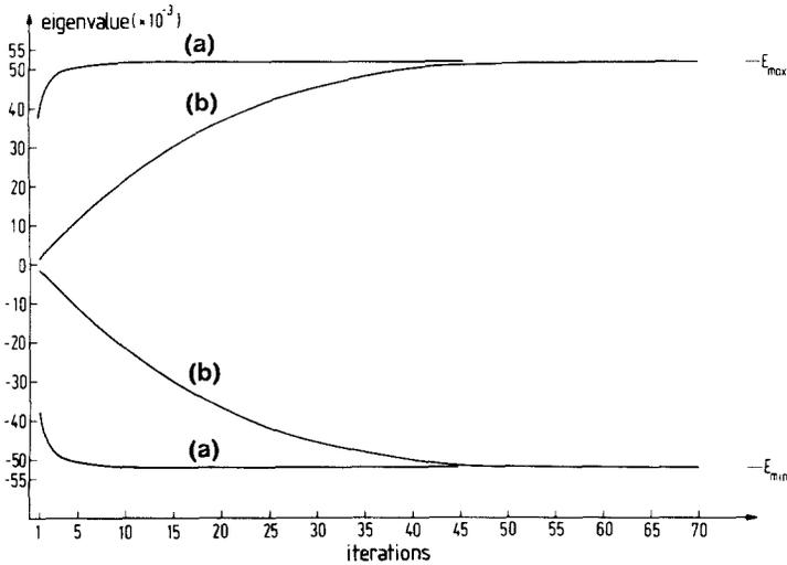
Fig. 1. Comparison of two trial states for the even  $M$  band.
