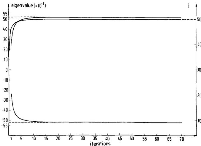
**Fig. 3.** Iteration scheme for the Hamiltonian (5.2); iterations versus energy (left axis) and quasispin (right axis).
